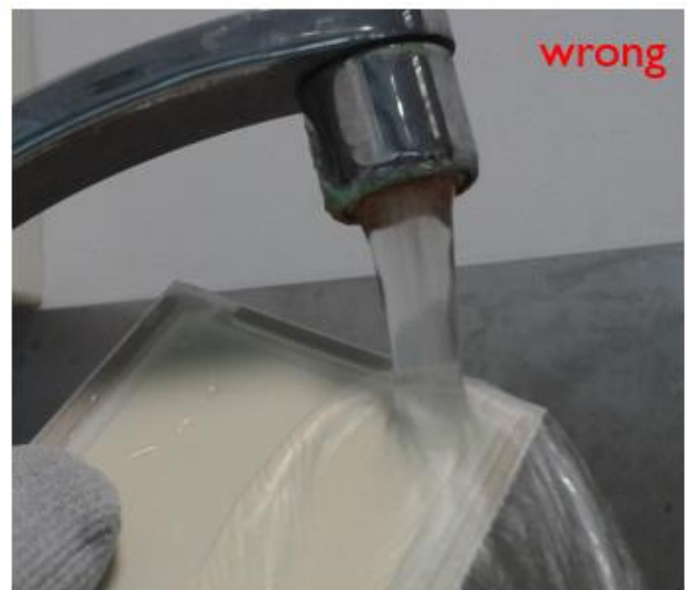
Left: Do not fold the device. Do not bend it with a radius smaller than specified. Right: Do not clean the OLED with water.
